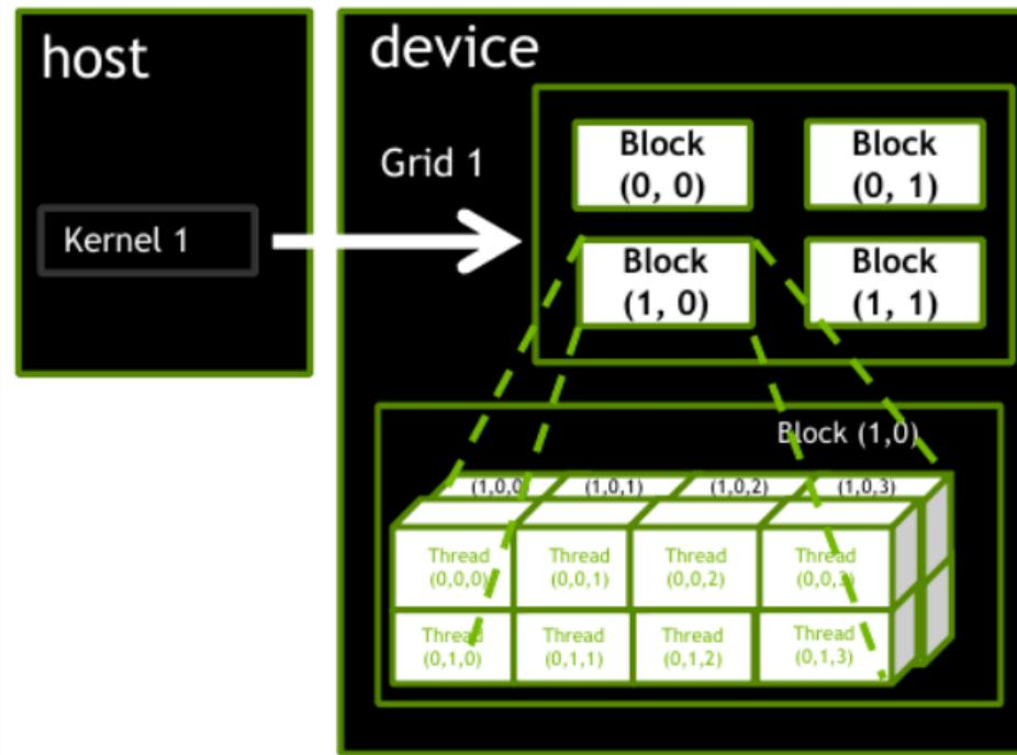
A 2D grid of blocks, with 16 threads per block in 3D (source: NVIDIA DLI).
