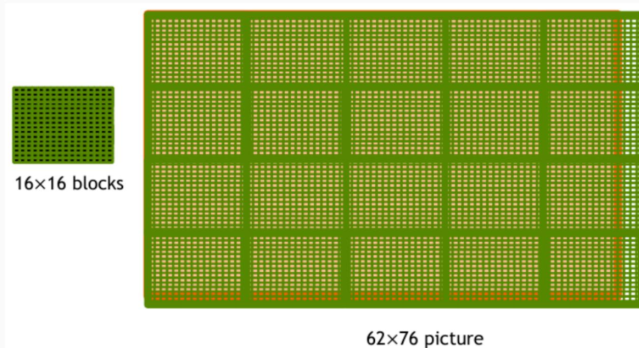
A 2D grid of blocks with 16 threads each in 2D (source: NVIDIA DLI).
