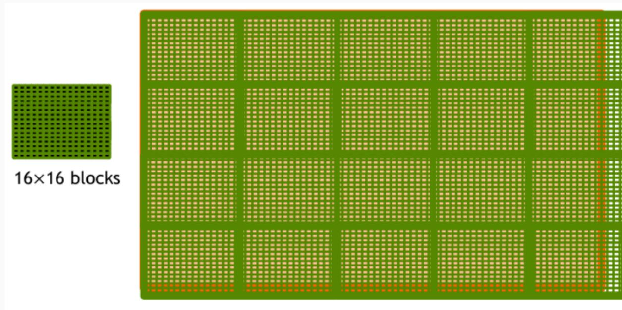
A 2D grid of blocks with 16 threads each in 2D (source: NVIDIA DLI).
